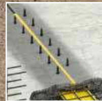
Leaking Movement Joints
